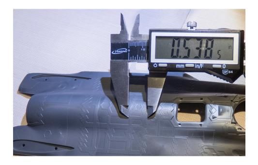
In ecal2, click to select the outline then right click -> Transform -> Scale and change the height to the caliper measurement. Make sure keep proportions id checked. The reason is the scale gets a little bigger along the way. It's the correct shape...it just needs to be proportionally scaled back.
