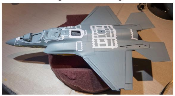
The F-35B had some unique challenges with masking some of the sawtooth shapes on the fuselage. Sure you could mask them the old fashion way with a roll of masking tape, a straight edge, and an X-acto knife. But the drawbacks are many such as cutting and re-cutting small pieces of masking tape along with the biggest problem of possible damage to the model from too much handling.
