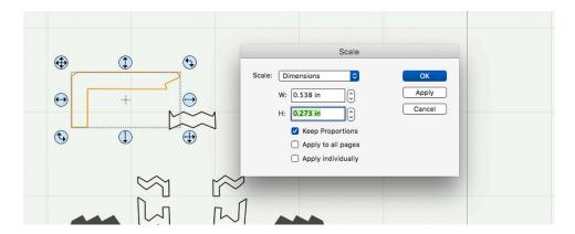
If there's a duplicate section on the other side of the model, make a copy of the image. Select the copy, right click, Transform -> Flip Horizontal (Mirror)
