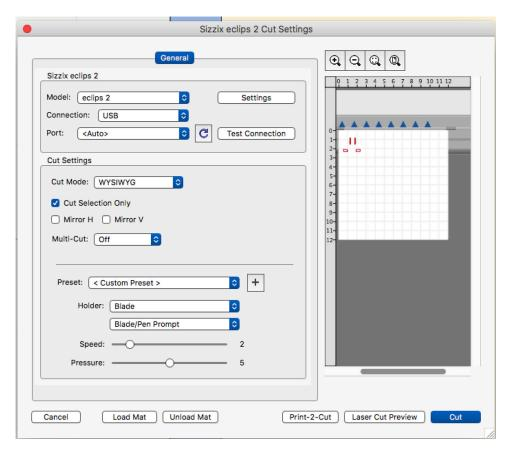
Set the speed to 2 so the blade makes a clean cut. Set the pressure to 4 or 5. Depending on how many shapes you selected, it may take the cutter several minutes to finish. Below is a picture showing the removal of the cut shapes from the mat and applied to the model
